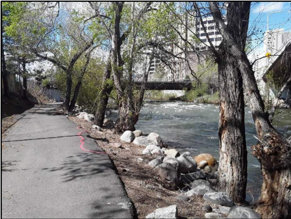
Photograph A-9. Lake Street through Brodhead Park. City of Reno, L63, L64, L66, L67, L68, L69. Steep actively eroding slopes with prominent invasive species (tree of heaven) (L64).
